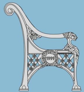
The 580 design of seat is quite unusual as it is nearly an all cast construction. The back panel of the seat is a trellis type casting. Timber slats are only used on the seat base.
